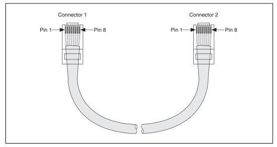
Figure 11. Ethernet Connector Pinout
